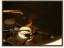
by high frequency, induction, or a torch to melt the metal, while the arm is in a cocked position. When the precious metal is at critical temperature, the centrifuge is released and metal is slung from the crucible at high velocity, filling the flask before it spins to rest.
