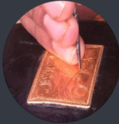
Traditional designs are drawn on the gold surface with a pointed steel scriber.
