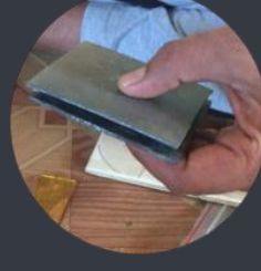
Together they are transferred to open crucible filled with, temperature high enough to fuse gold and glass (below gold melting point)
