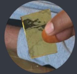
Transparent and bubble free glass cut into a shape corresponding with that of a decorated foil.
