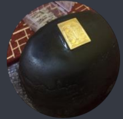
Raar (lac) is warmed and the metal is fixed onto it
