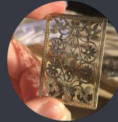
The finished pierced work (the waki patti) is heated and stripped from the lac
