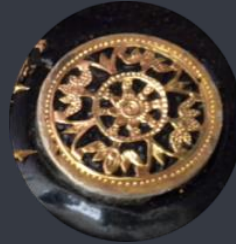
Leaving frame intact, the internal background of the design is removed by piercing
