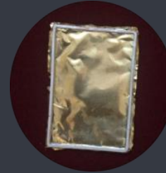
Soldering gold 40 gauge sheet to silver frame
