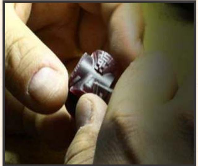
With the advent of high frequency melting and a host of other technologies, jewelry casting is more dynamic than ever. Most jewelry casting is done through the lost wax process, whereby models created through wax carving, growing, or printing are encased in a plaster- like medium known as investment. The investment is heated to extreme
