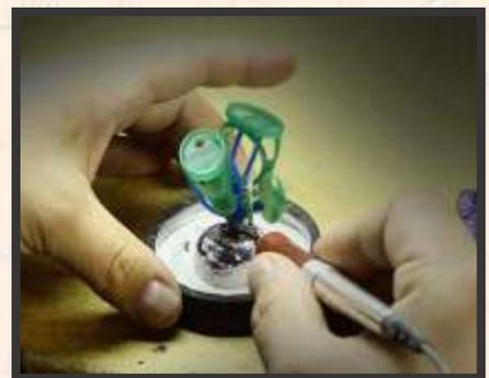
temperatures to incinerate the material, creating an impression of the desired form. The intricate cavity is then filled by molten precious metal.
