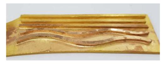
Note that the solder has flowed through the entire strip in a clean and uniform way, without excesses and without pores.
