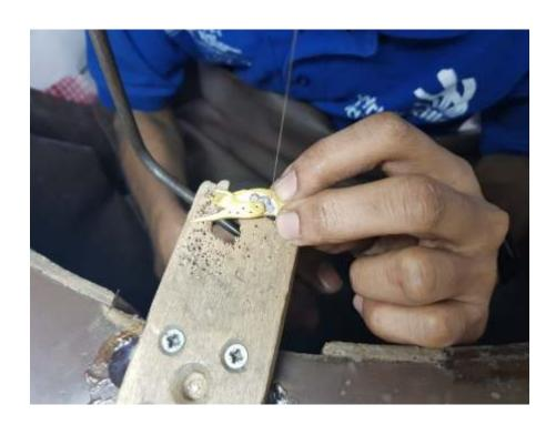
Make the correct drilling, using the drill in 90 degrees and saw it exactly as the technical drawing demonstrates.
