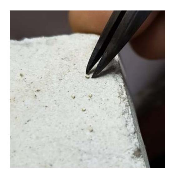
Knowing this very important tip, after positioning each tube in the same way as the technical drawing, a solder ball is placed on the side at the contact between the plate and the small tube and we do the welding.
