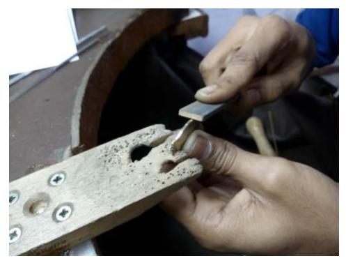
Sand the pieces in one direction only as much as possible in a way the pieces have a good look when the process is finished.
