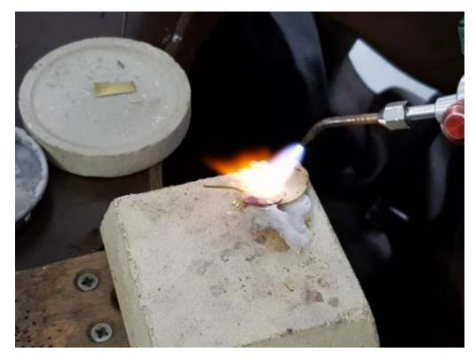
Put the pieces together to be soldered correctly. Use iron wire when necessary to hold the parts. Sometimes the tweezers can be used to hold two plates. Make the solder balls as explained previously, so that the solder flows well.
