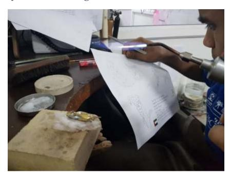
Properly solder the bezel from module 3 on module 2. If necessary, use iron wire to be able to hold both parts in place. Always remember to make solder balls to solder the parts.
