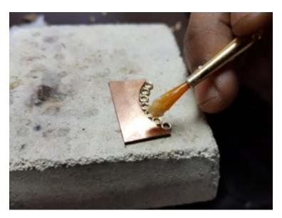
Use only the minimum necessary solder flux between the rings so that when you pass fire they will not move when the flux gets hot. To weld them between one another, make solder balls again before placing the soldering pieces between the rings. Use small pieces of soldering, just what is needed for welding, without over soldering the place.
