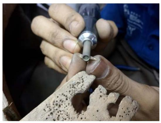
Use the sanding rollers on the shaped parts to give them a faster, smooth and uniform finishing. Use the sanding splints where the sanding rollers are not a good option, as on flat pieces (or parts).
