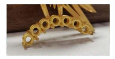
Always place the soldering where it can be sanded or where it will not appear in the overall look of the piece. Remember of the good looking piece tip.
